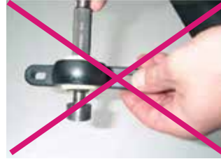
Inadequate test equipment; plug gauge too short
