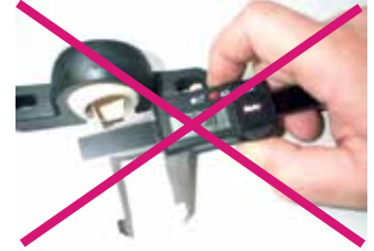
Wrong test equipment; caliper
